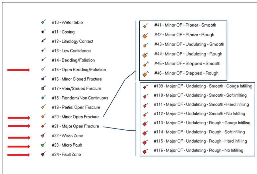
Figure 2. Typical structure classifications for geological structures (left) and with categories expanded for geotechnical purposes (right).
