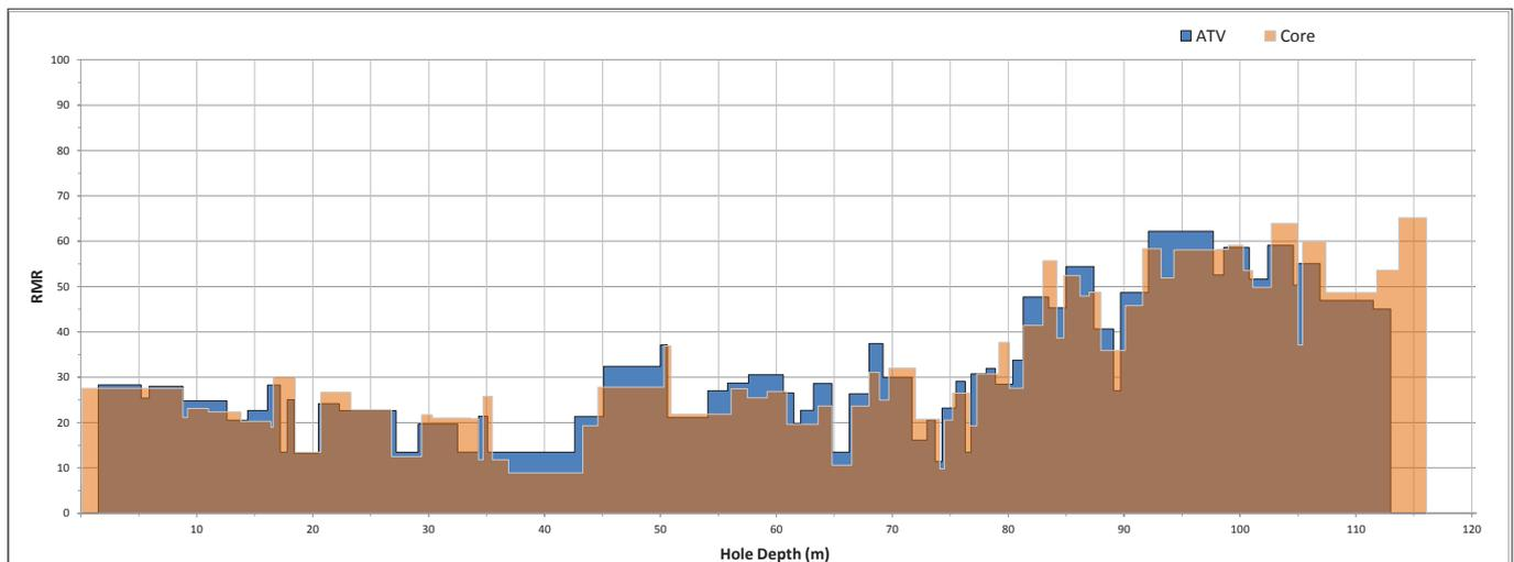
Figure 5. Rock mass rating values derived from logged drill core and acoustic televiewer tool data.
