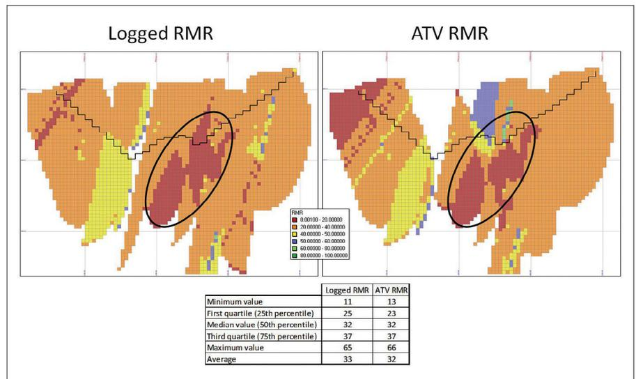
Figure 6. Rock mass model sections showing estimated rock mass rating values for logged versus acoustic televiewer tool data.
