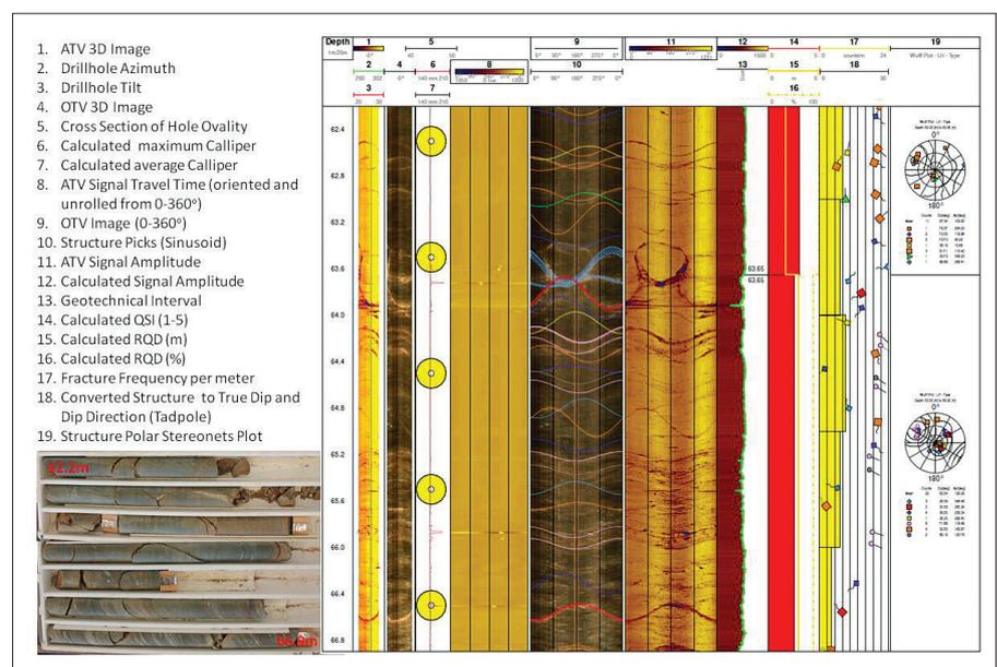
Figure 1. Image from acoustic and optical tools and geotechnical interpretation compared with drill core photo.
