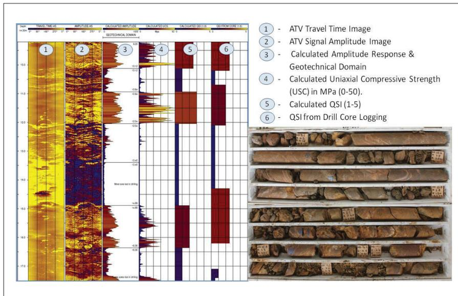
Figure 4. Image from acoustic televiewer tool and geotechnical interpretation compared with drill core photo.
