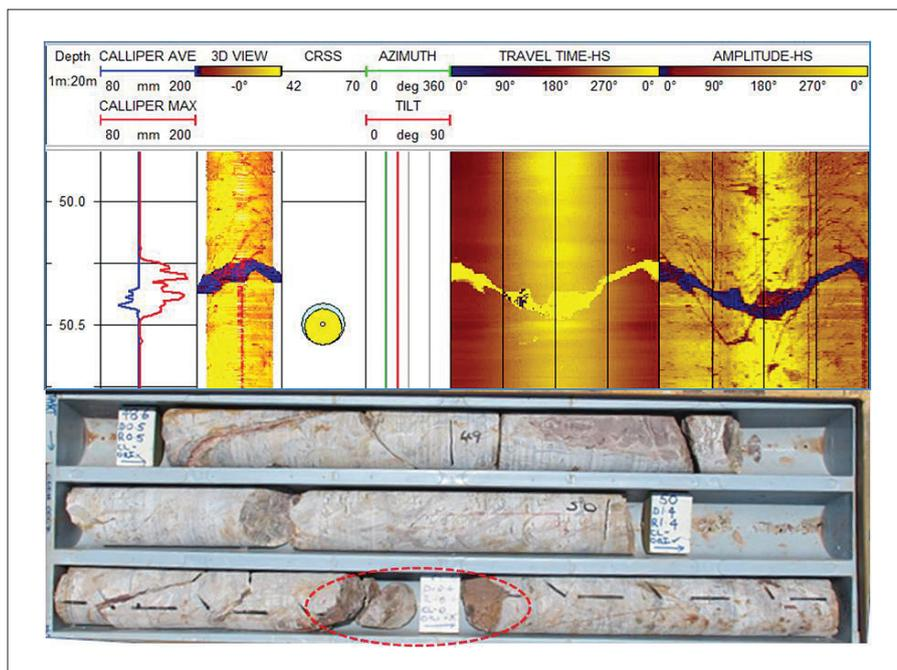
Figure 3. Example of a rough and undulating joint identified in acoustic viewer tool data and drill core.
